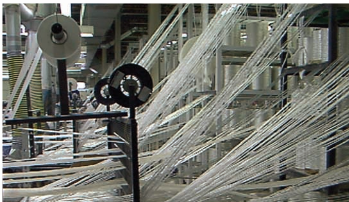
Glass strands are being organized prior to entering the pultrusion die.
